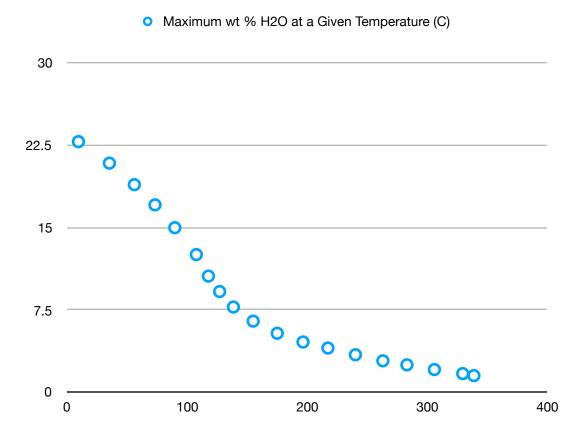
Please note that the above curve is for pure molecular sieve. The carrier material we use to mold the getter reduces the maximum capacity to ~ 11 wt%.
